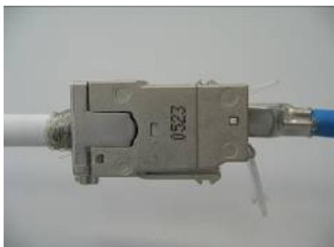
Fig 11 : Screen transfer Plug/Jack
