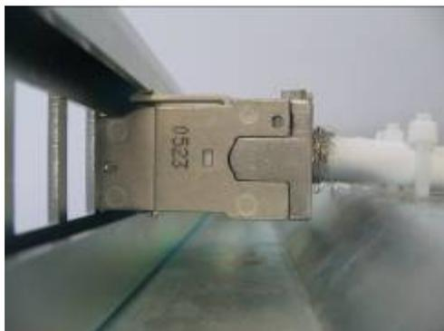
Fig 10: Screen transfer panel and mounted shielded jack
